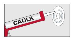
Caulk may be applied to the back of the Dry Seal Pipe Collar when using over grout lines or irregular walls.
