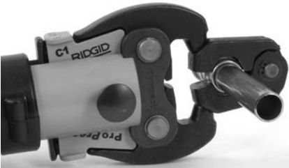
Figure 10 – Attaching Actuator to Press Ring
