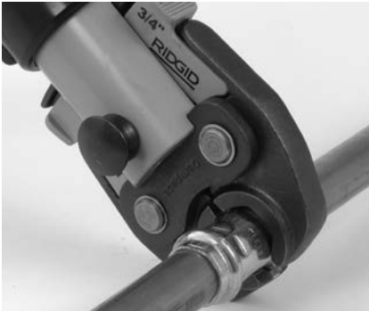
Figure 7 – Placing Scissor-Style Jaws Around Fitting
