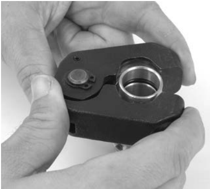
Figure 9 – Installing Press Ring onto Fitting
