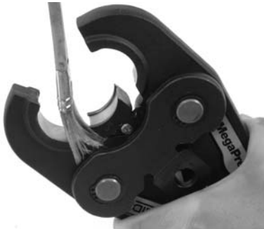
Figure 11 – Cleaning Segment Area of MegaPress Jaw
