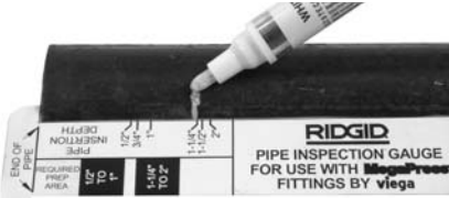
Figure 5B – Marking the Pipe Before Inserting Into Fitting Using RIDGID® MegaPress® Pipe Inspection Gauge
