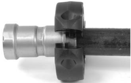
Figure 9 – Opening the MegaPress Jaw set and Placing Around Fitting
