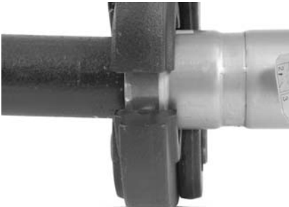
Figure 8 – MegaPress Jaw Set Square To Fitting and Tubing
