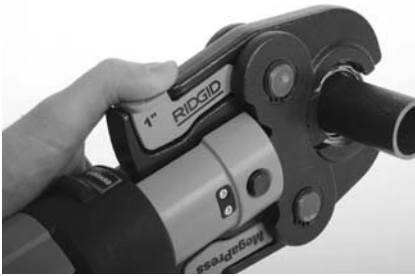
Figure 7 – Opening the MegaPress Jaw set and Placing Around Fitting
