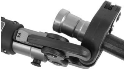
Figure 10B – Placing V2 Actuator Into MegaPress Ring Pockets At An Angle For Additional Clearance
