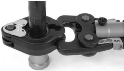
Figure 10A – Placing V2 Actuator Tips Into MegaPress Ring Pockets
