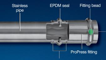
Unpressed connection with the Smart Connect feature allows liquids and/or air to pass by the sealing element during pressure test.
