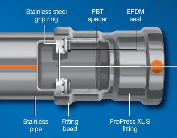
The stainless steel grip ring is pressed, forcing the grip ring teeth against the tube, making a highstrength connection.
