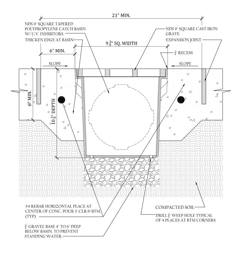
• GRATE TO BE ATTACHED TO CATCH BASIN WITH SCREW PROVIDED AT TIME OF INSTALLATION.
