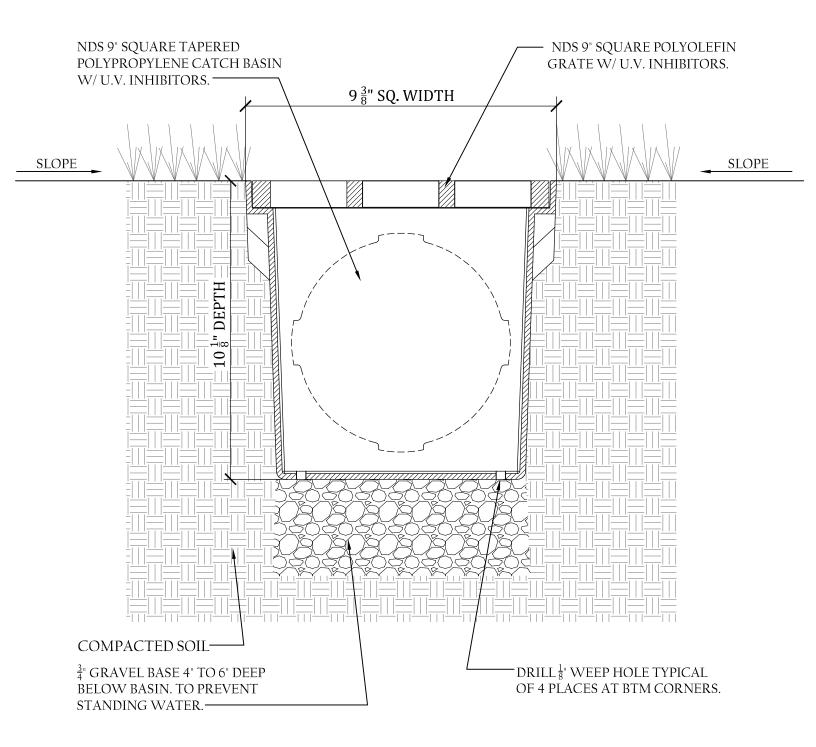
• GRATE TO BE ATTACHED TO CATCH BASIN WITH SCREW PROVIDED AT TIME OF INSTALLATION.
