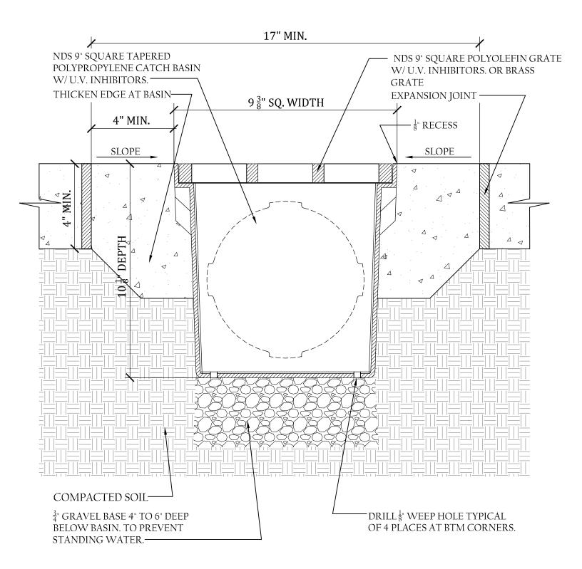
• GRATE TO BE ATTACHED TO CATCH BASIN WITH SCREW PROVIDED AT TIME OF INSTALLATION.
