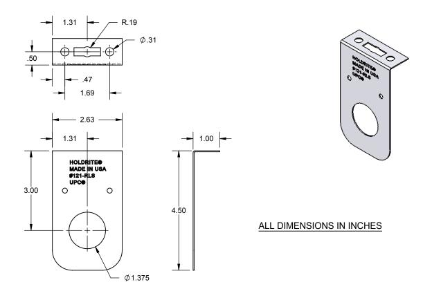
The HOLDRITE® #121-RLS is a 20 gage galvanized steel bracket that support a single line of 1/2", 3/4" or 1" Copper, PEX or CPVC tubing at 3" center line height. The hole pattern on the  $90\,^\circ$  base allows for attachment to any flat surface. The bracket can also be suspended by 1/4" or 3/8" threaded rod.
