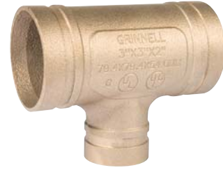
FIGURE 621 REDUCING TEE GROOVE X GROOVE X GROOVE CAST
