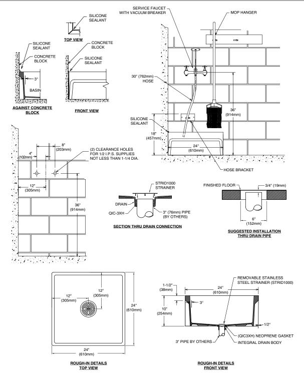
**Installation Note:** QIC32 Quick Drain Connector for 2" pipe or QIC3SN Quick Drain Connector for cast iron soil pipe must be ordered separately.
