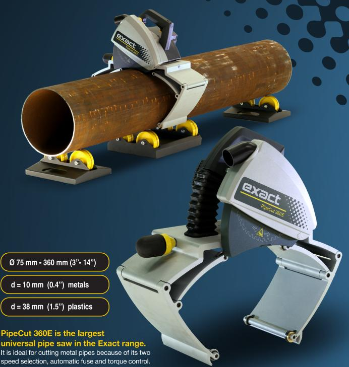
speed selection, automatic fuse and torque control. It is also suitable for cutting plastic pipes because it can cut very thick wall pipes and it can be attached to a vacuum cleaner. Because of its robust design and construction plus large capacity it is ideal for heavy-duty use.
