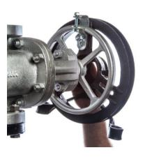
3. Put a washer (if included) on a bolt, pass the bolt through the slot in the chainwheel from the front, pass through both sides of the strap, and fasten loosely with a lock washer (if included) and nut. Repeat to fasten the remaining U strap.
