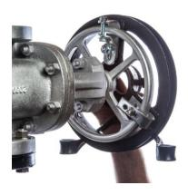
4. Center the chainwheel and tighten the nuts securely.
