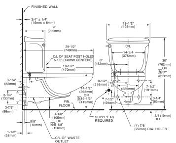
NOTES: WASTE OUTLET SEAL RING MUST BE NEOPRENE OR GRAPHITE-FELT (WAX RING NOT RECOMMENDED) SUGGEST 1/16" CLEARANCE BETWEEN FACE AT WALL AND BACK OF
